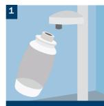
Turn off delivery system, remove and empty the water bottle.
