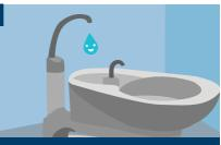
Run solution through the Dental Unit Waterlines (DUWL) until you start to see blue water from the tubing and cuspidor cupfill (where relevant).
